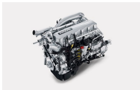
The highly efficient and powerful 12.9 liter PACCAR MX-13 engine features sophisticated technologies like common rail injection, a variable geometry turbo and exhaust gas recirculation.
